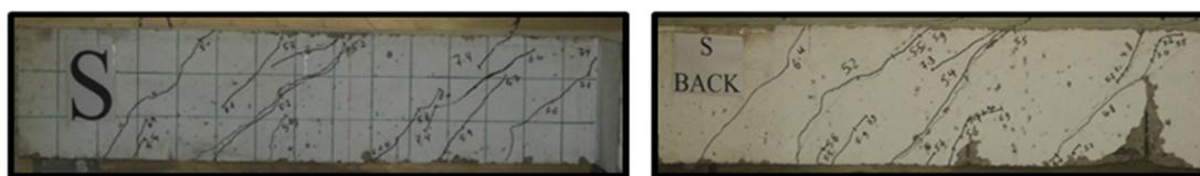
a) Crack pattern for the solid specimen
